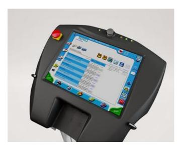
OptiCycle, a plug-in for the Sepro Visual control, can envision the entire robot cycle, then break the program down into its component elements. Within each element, it offers programming instructions and best practices to guide the operator.
