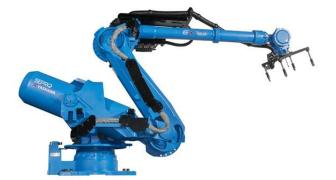
The 6X-400 6-axis articulated-arm robot, the product of a recent manufacturing partnership with Yaskawa Motoman, has a 4m reach and can carry a maximum 120-kg payload. Download a high-resolution image at: <u>http://tinyurl.com/hbl8vap</u>
