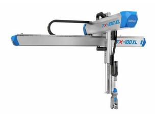
The new 7X-100XL has a 5m horizontal beam, a telescopic vertical stroke of 3.2m and a maximum payload of 100 kg. Download a high-resolution image at: <u>http://tinyurl.com/jevt5ru</u>
