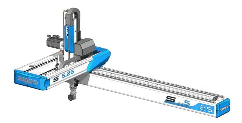
Being shown in Mexico for the first time, the 3-axis Sepro S5-25 Speed, was developed for molders seeking a high-speed robot to serve injection-molding machines from 120 to 450 tons. Download a high-resolution image at: <u>https://tinyurl.com/SRO-S5-25Speed</u>
