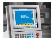
Open Integration from Sepro allows the robot control interface to be presented on the molding machine HMI. Download a high-resolution file at: https://tinyurl.com/OpenIntegration
