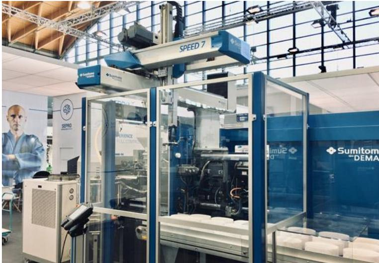
*One of the two automation cells on the Sepro stand will feature a Sumitomo Demag molding machine equipped with an SDR Speed 7 robot. Made by Sepro especially for sale with Sumitomo Demag machines, this robot is capable of getting in and out of the mold space in under 1 sec. Download a high-resolution file: <https://tinyurl.com/SRO-Speed7>*
